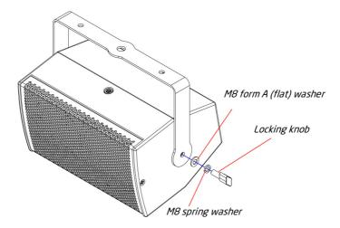
Ensure that the washers are in the correct order - form A (flat) in contact with the frame, and then the spring washer between the flat washer and the locking knob. Tighten the knobs on both sides to lock the desired angle for the EMS-51.
