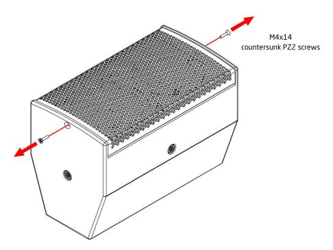
2. To replace the grille, position the grille on the front of the EMS-51 and ensure the threaded fittings on the grille are lined up with the mounting holes - gentle pressure may be required. Replace both of the M4x20 countersunk screws and ensure they are both are started in their threads before beginning to tighten. Ensure they are all tightened evenly so that the grille sits straight and flat and does not rattle. Be careful not to over-tighten as this will distort the grille.
