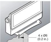
Two quarter-turn brackets are supplied with the fixture if it is to be flown above the ground. Remove the floor stand/base and rig the Q-7 to a support truss or structure using the supplied brackets and suitable clamps.
