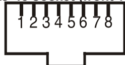
RJ-45 socket (front view):
