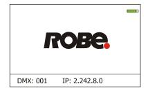
The green icon at the top right corner of the screen indicates the level of the display battery charging. If the whole icon is green, the battery is fully charged while the red icon indicates exhausted battery. The battery charges during fixture operation, its charging lasts cca 6 hours.
